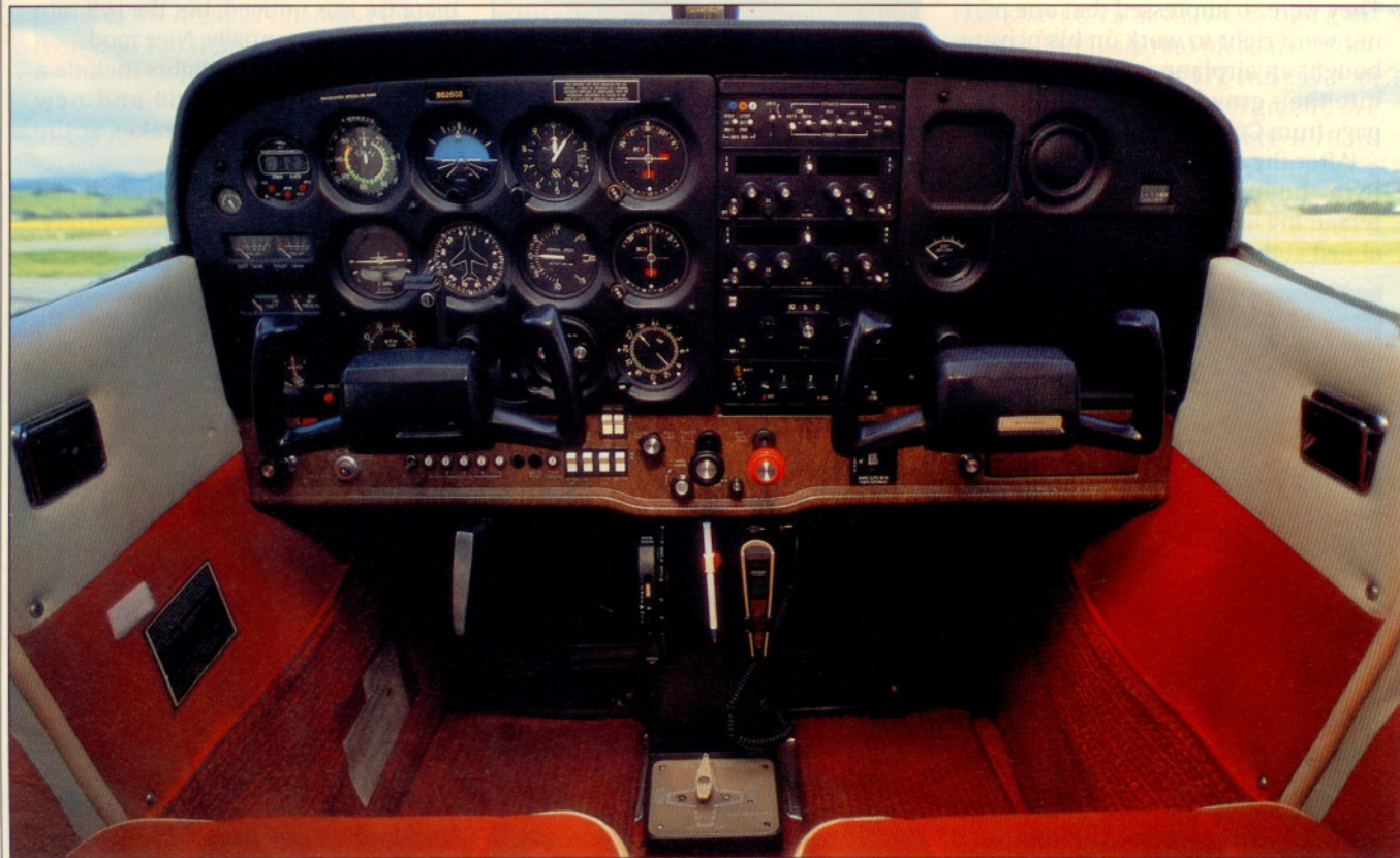
Ron Sieg (above) opted for a full IFR panel in his 1982 Skyhawk. His 172P, also shown on p. 58, carries the last model designation.
